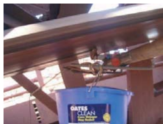
The measurement shows the carryback on the belt
