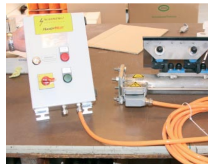
A controller measures the temperature
