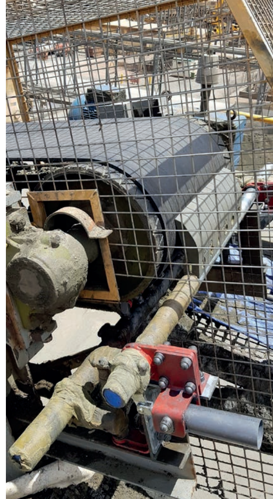
Sturdy HOSCH scrapers in service on a belt conveyor at the opencast gold mine in Kalgoorlie (Western Australia).
