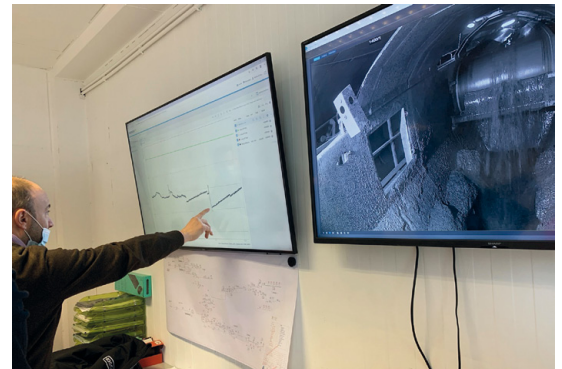
Fig. 5: Mattia Corna conducting a visual inspection of sensor data in the control room (left) and video stream from the belt head and transfer point (right)
