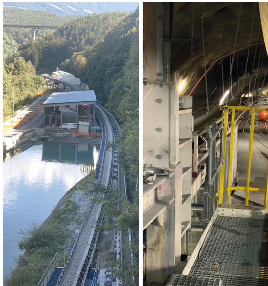
Fig. 1: Long distance belt installations above and below ground – a pair of conveyors running inside the tunnel
